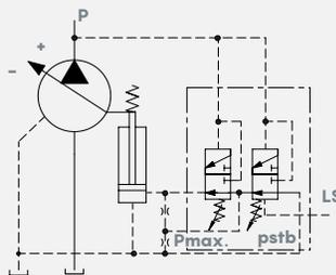
P-LS control is the traditional Load Sensing control, aimed to keep a constant pressure margin through the main control valve.
