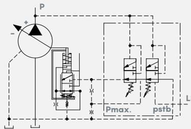
The P-LS-TC adjusts the pump displacement based on pressure to ensure that the absorbed torque does not exceed the set value, protecting the motor from overloads. If set lower, the Torque Control will limit the maximum operating pressure to a value below the standard pressure control setting (280 bar - 4050 psi). When ordering the torque limiter, please specify the required torque value (e.g., 100 Nm - 73.75 lbf·ft) or the required power and speed (e.g., 15 kW at 1300 rpm).
