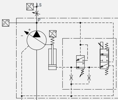
ALS-FC control works with a constant synchronization with P and LS pressure sensors, angle sensor and ECU.
