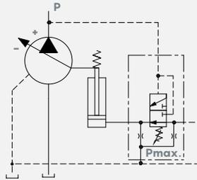
The pressure control regulates the maximum pressure at the pump outlet within the adjustment range of the variable pump. The pump supplies only the necessary amount of hydraulic fluid to meet consumer demand. If the operating pressure exceeds the set value at the pressure relief valve, the pump displacement is set to minimum.
