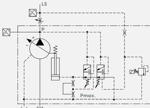
ALS-MC control works with P and LS sensor in closed loop with ECU. This control modifies the load pressure signal on the standard LS control: it's possible reduce the operating standby. Additional torque control strategies can be added.
