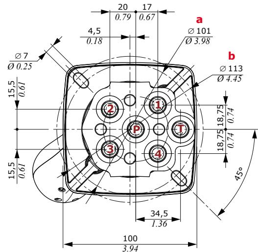
NOTE: normally the pilot control valve is supplied with the handle oriented towards ports nr. 3/4
