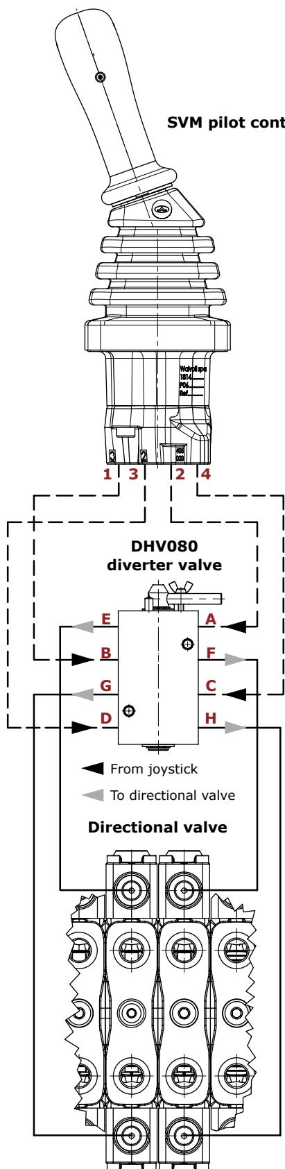
**Joystick movement****Diverter valve in position 1**
