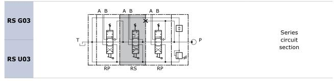
When the spool is operated it intercepts the switch gallery by diverting the flow of oil to service port A or B. The oil that flows back from the actuator is carried to the switch gallery thus making it available to the service ports downstream from the series section. The pressure drop downstream is added to the pressure drop of the section itself.
