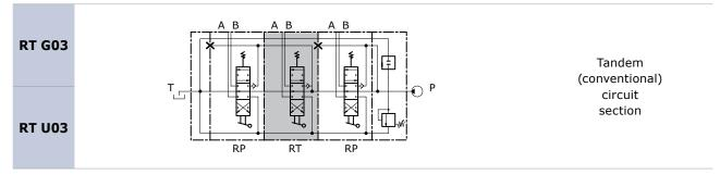
When the spool is operated it intercepts the switch gallery by diverting the flow of oil to service port A or B. The Tandem circuit is powered by the switch gallery thus permitting the use of just one work section at a time. The section downstream from the tandem section that has been actuated does not operate, the upstream section has priority.
