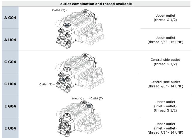
NOTE: code "E" on outlet section obliges to choice E on inlet section.
