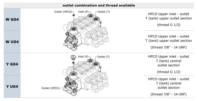
NOTE: code "W" or "Y" on outlet section obliges to choice E on inlet section.
