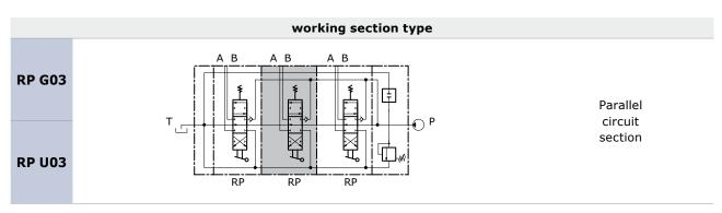
When the spool is operated it intercepts the by-pass gallery by diverting the flow of oil to service port A or B. If two or more spools are actuated at the same time, the oil will power the service port that has the lower load; by throttling the spools, the flow of oil can be divided between two or more service ports.
