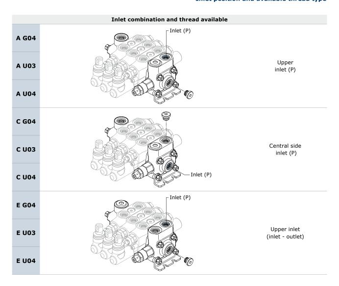
NOTE: code "E" on inlet section obliges to choice "E", "W" or "Y" on outlet section.
