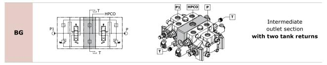
The section in question allows the flow of oil of the two pumps to be piped in two outlets: HPCO for powering another directional control valve, T for discharge of the work ports. In order to obtain this, the two T need to be linked.
