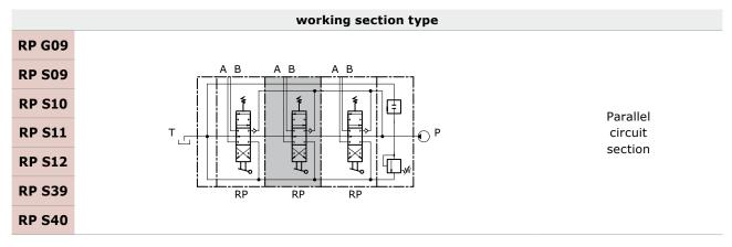
When the spool is operated it intercepts the by-pass gallery by diverting the flow of oil to service port A or B. If two or more spools are actuated at the same time, the oil will power the service port that has the lower load; by throttling the spools, the flow of oil can be divided between two or more service ports.
