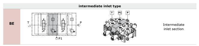
The intermediate inlet section is driven by two pumps (P + P1). The downstream elements can be set to a lower pressure than the upstream ones by adjusting the pressure relief valve of the intermediate section in question.
