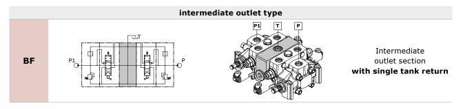
The above outlet section allows the flow of oil of the two pumps and the tank ports to be piped to a single outlet T.
